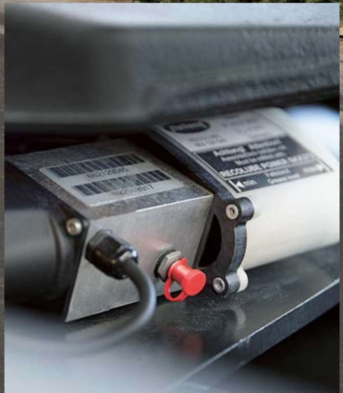
With the RECOLUBE automated lubrication pump, it is no longer necessary to lubricate fifth wheels manually.
